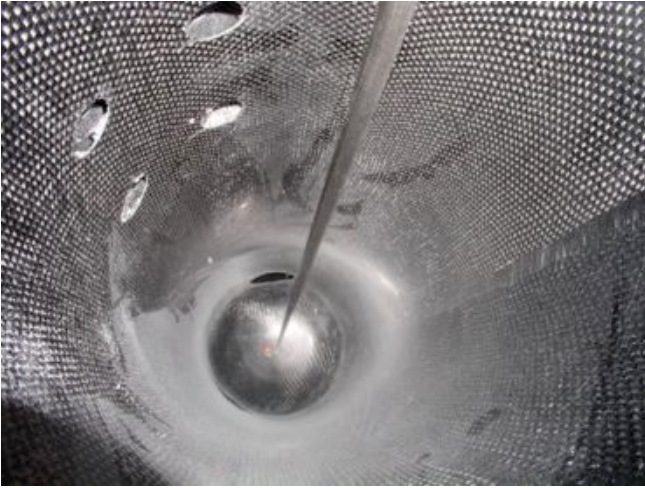
Picture 2 and 3: making the hole (internal and external view) For making the hole in used a long drill in diameter of 5 or 6mm.
