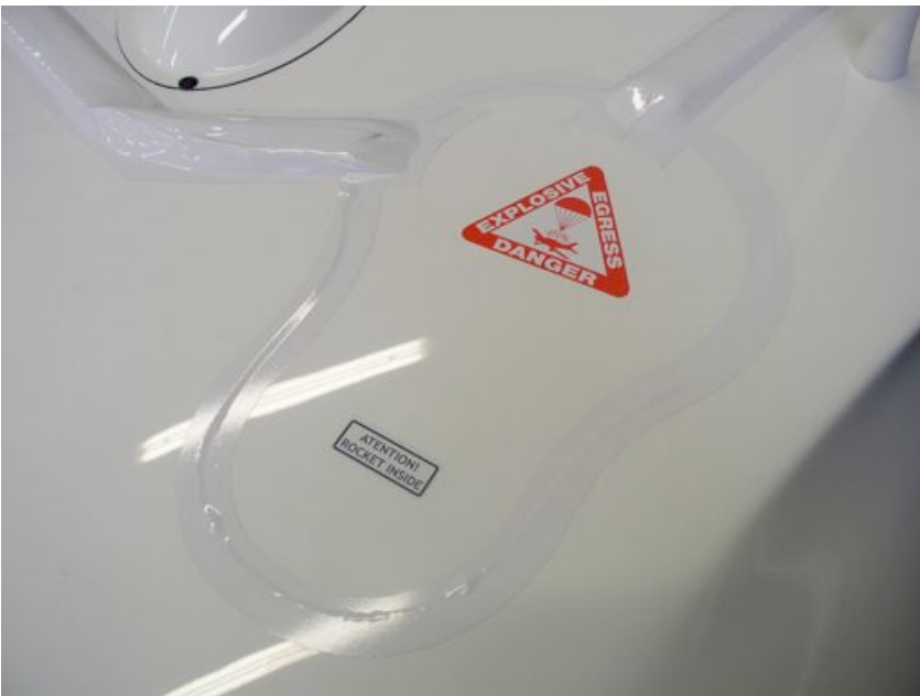
Picture 10: Insulation tape around the container cover
