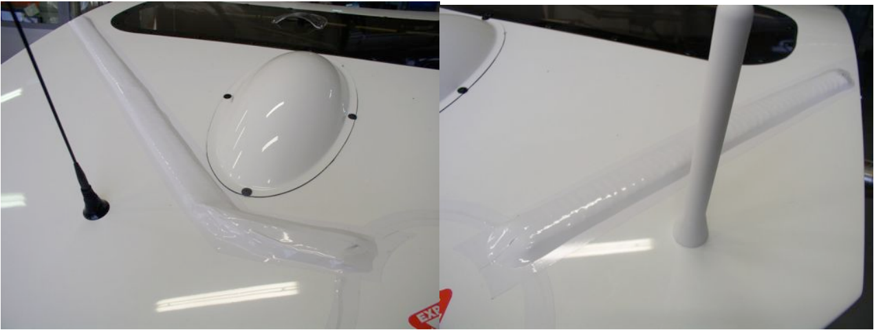
Picture 8 and 9: insulating tape on the main parachute rope
