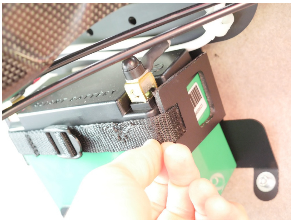
Figure 2: Fore battery installation – tearing away the strap's loose end
