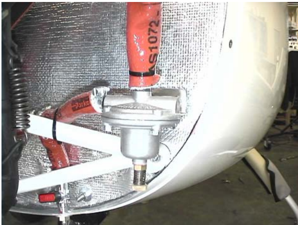
50 ccm version gascolator as mounted on aircraft ( affected )
